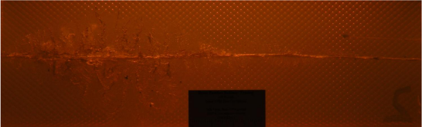
Figure 10. Side View of 2200 ft/sec impact gelatin block
