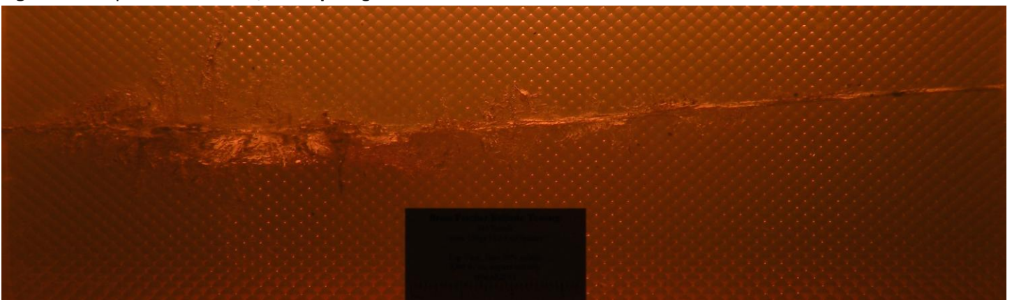
Figure 11. Top View of 2200 ft/sec impact gelatin block
