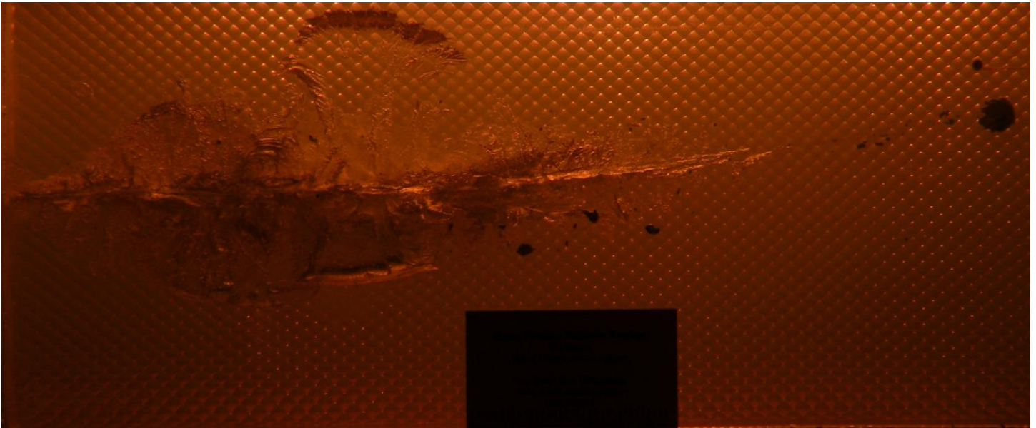
Figure 5. Top view of 2461 ft/sec impact gelatin block
