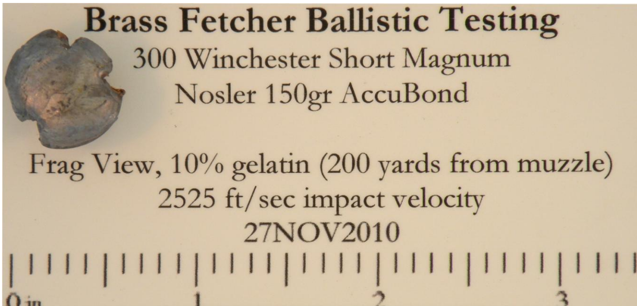
Figure 12. Projectile view of Shot 3 recovered fragments
