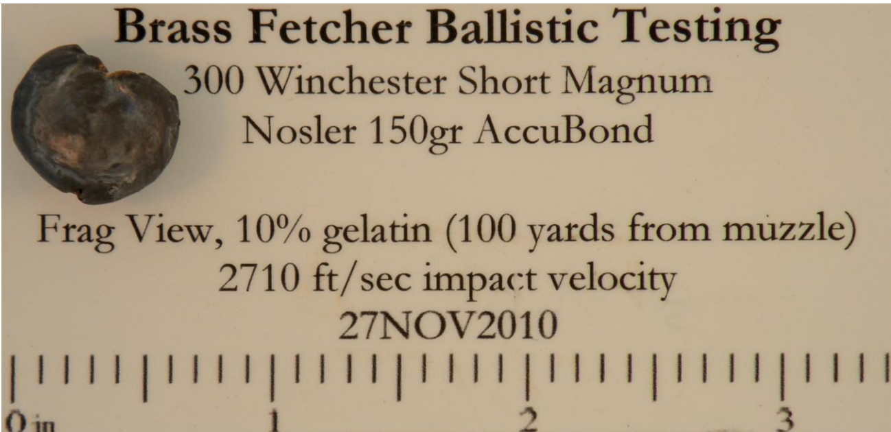
Figure 9. Projectile view of Shot 2 recovered fragments
