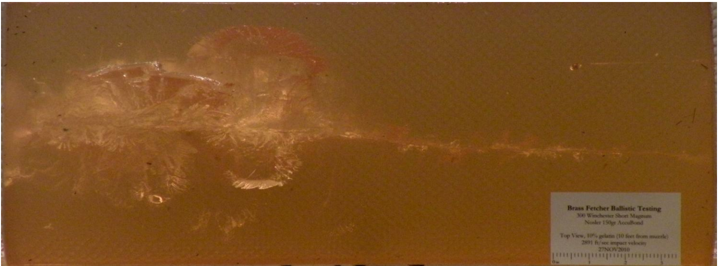
Figure 5. Top view of Shot 1 gelatin block
