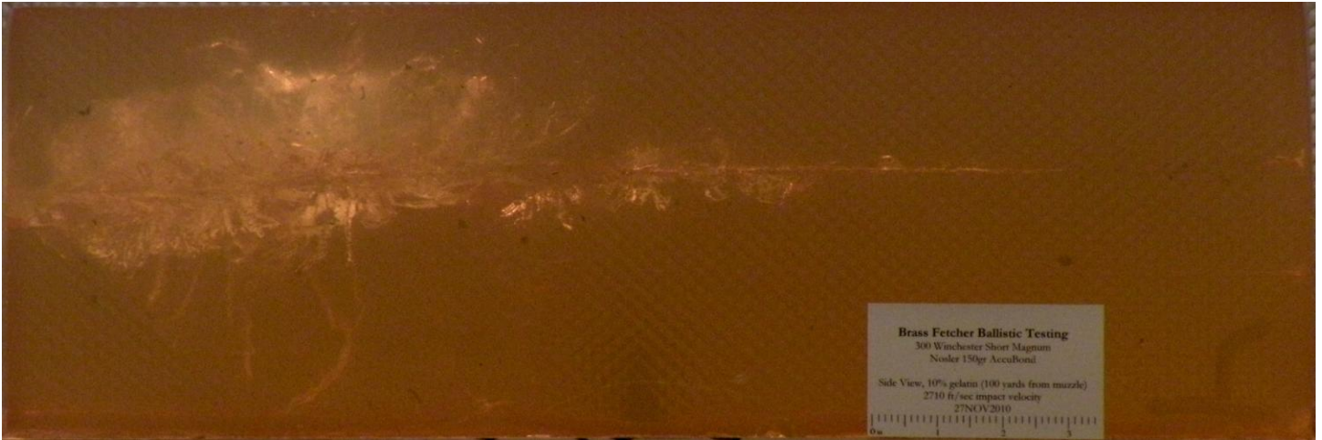
Figure 7. Side view of Shot 2 gelatin block
