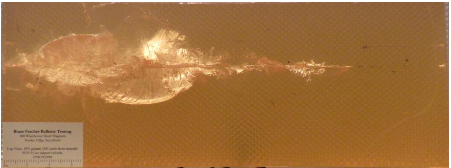
Figure 11. Top view of Shot 3 gelatin block
