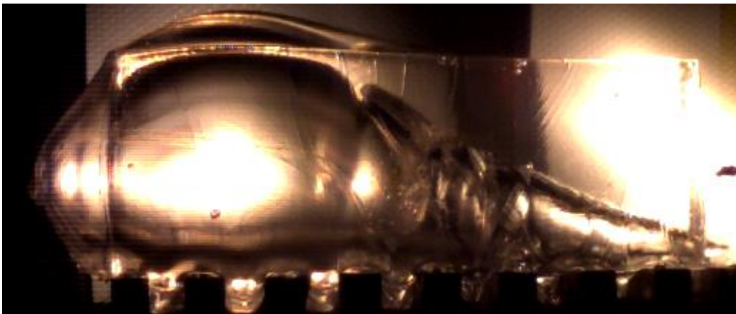
Figure 4. Barnes 55gr TSX impacting Clear Ballistics™ ballistic gelatin
