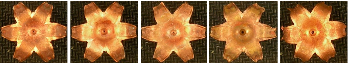
Figure 7-11. Cor-Bon 115gr +P DPX recovered bullets (Shots 1-4 through bone; Shot 5 bare gelatin)
