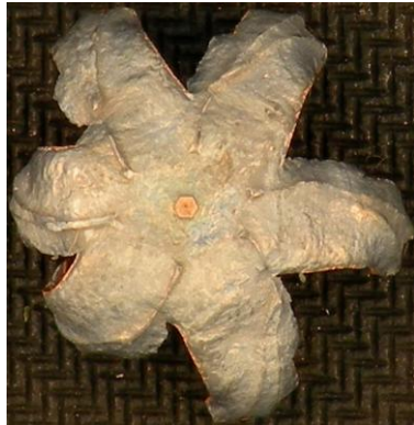
Figure 24-27. Speer 124gr +P Gold Dot recovered bullets (Shots 1-3 through bone; Shot 4 bare gelatin)
