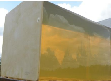
Figure 1. Bone simulant plate and ballistic gelatin block
